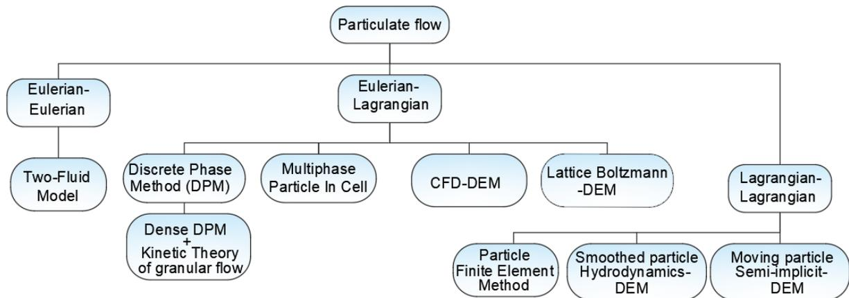
Figure 2. Different approaches and their corresponding models for particulate flow modeling
